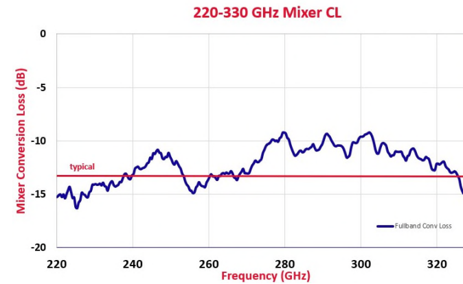
Fig 4 : 220-330 GHz Intrinsic Mixer Conversion Loss (SSB)
