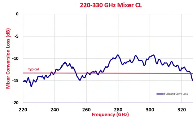
Fig 4 : 220-330 GHz Intrinsic Mixer Conversion Loss (SSB)
